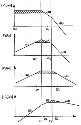
Given any set  $|V_i(j\omega)|$  of basis functions, then it is always possible to find a new set  $|V_i(j\omega)|$  of basis functions with the same span but which satisfy (5.3) for a particular filter F and input spectrum  $\phi_n(\omega)$ . This can be achieved via the standard Gram Schmidt orthogonalization procedure (Goodwin et.al 1991). This amounts to taking a linear combination of the basis functions as follows:
